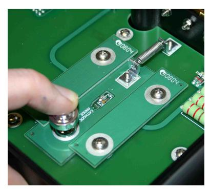
The DUT is installed by pulling back on the chrome knob, as shown below:
