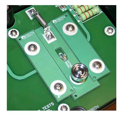
The anode pad must contact the left probe point, and the cathode pin must contact the right probe point.
